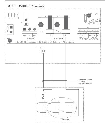
Figure 2.8 Battery Circuit Diagram
